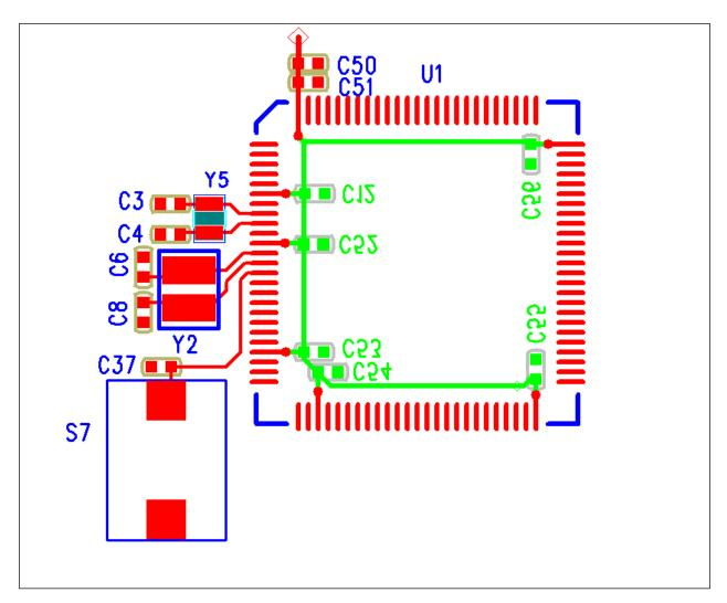
Figure 4-1 LQFP100 Package PCB LAYOUT reference diagram
