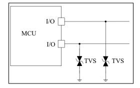
Figure 1-9 TVS connection on I/O pins
