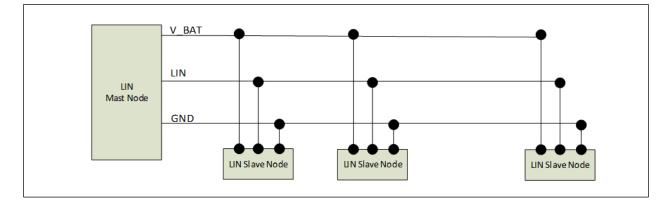
Figure 1-12 LIN typical interface circuit
