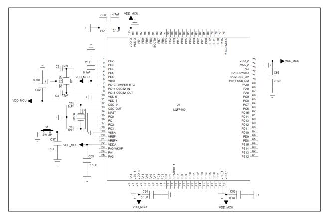
Figure 3-1 LQFP100 Package Minimum System Reference Design Schematic
