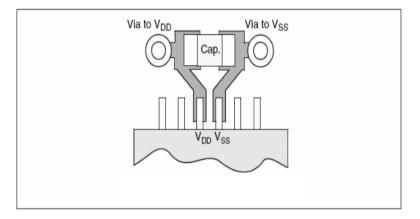
Figure 2-1 Typical layout of VDD/VSS pins
