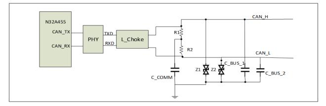
Figure 1-11 CAN typical interface circuit
