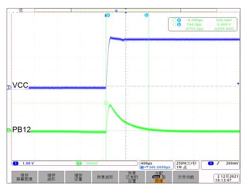
Figure 1-6 IO (PB12) waveform during power-on
