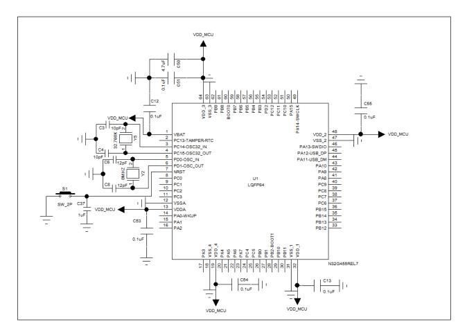
Figure 3-2 LQFP64 Package Minimum System Reference Design Schematic
