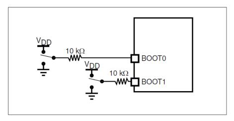
Figure 1-3 Implementation example of startup mode
