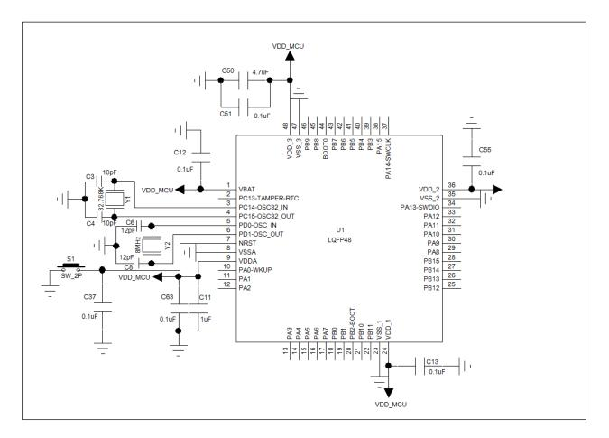
Figure 3-3 LQFP48 Package Minimum System Reference Design Schematic
