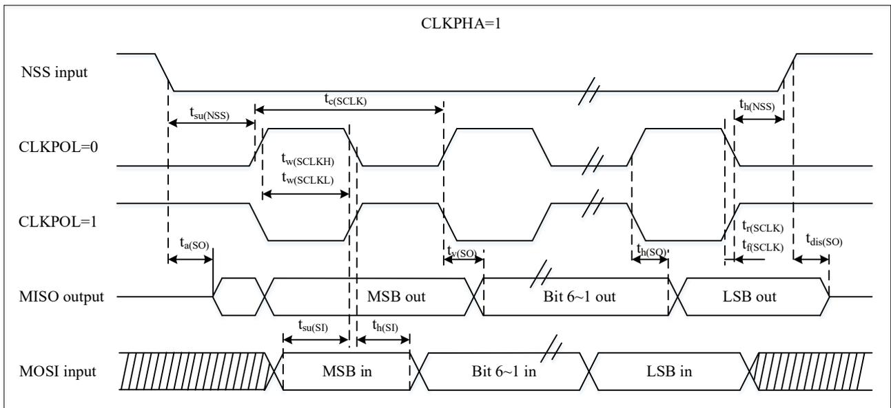
Note: <sup>(1)</sup> The measuring point is set at the CMOS level:  $0.3V_{DD}$  and  $0.7V_{DD}$ .
