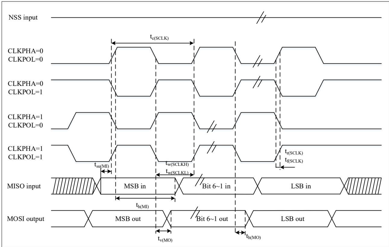
Note: <sup>(1)</sup> The measuring point is set at the CMOS level: 0.3V and 0.7V<sub>DD</sub>.
