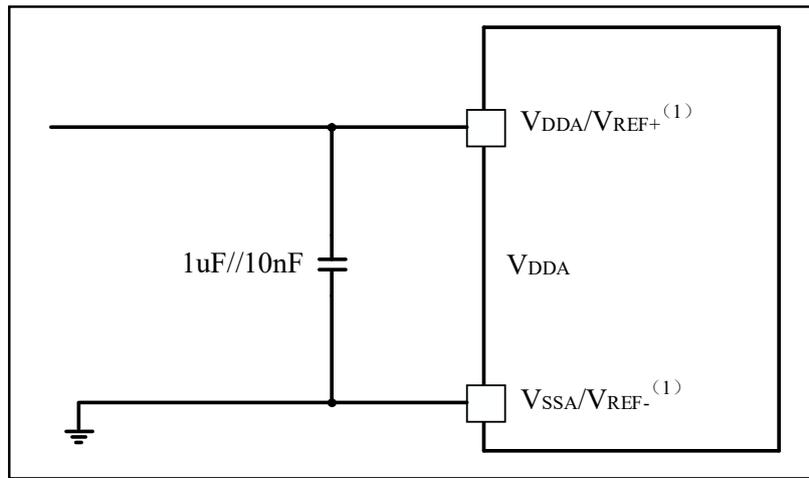
Note: <sup>(1)</sup>  $V_{REF+}$  and  $V_{REF-}$  are internally connected to  $V_{DDA}$  and  $V_{SSA}$ .
