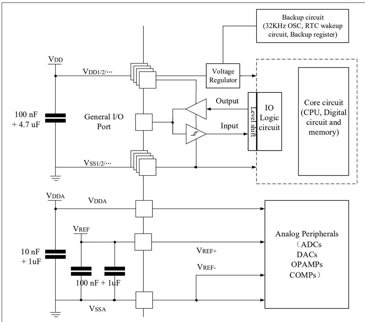
Note: Please refer to the hardware design guide for the capacitor connection method.  $V_{REF}$  is only available for ADC and DAC.
