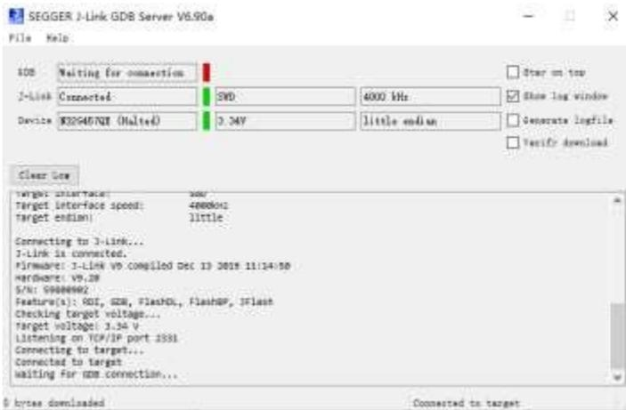
5. Under VSCode working environment, press "F5" or click "Run" -> "Start debugging". At this time, it can be seen that the label below turns green, indicating that gdb tool successfully connects to JLinkGDBserver.
